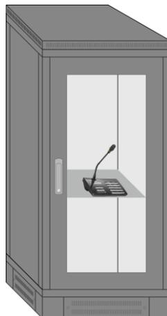
Fig. 2. Option 1 – microphone mounted in the DSO cabinet.
