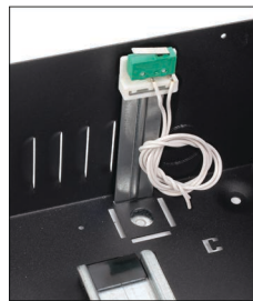
Tamper opening and detachment from the wall
