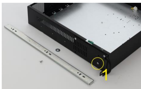
Remove the first M4 screw from ARAD enclosure
