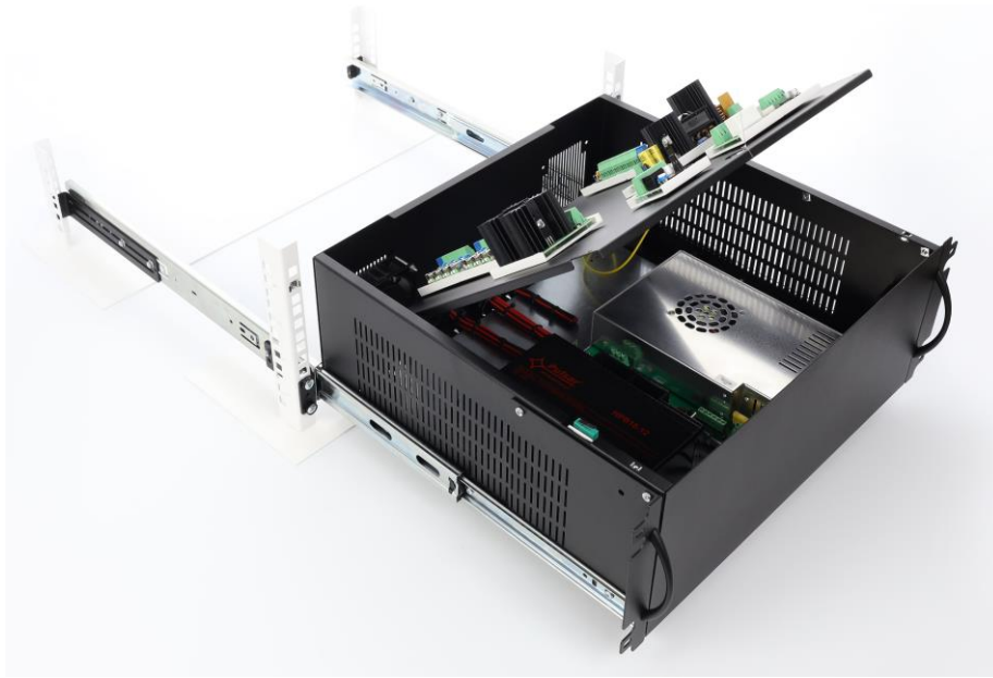
lide enclosure with sliders into the rails installed in 19" RACK cabinet
