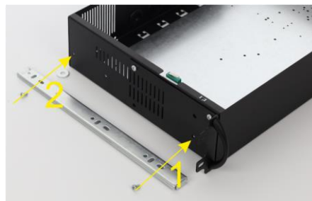
Fasten the sliders with two screws to ARAD enclosure (do not forget spacer washer under the second screw)
