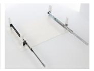
**3.2.** Remove slider and tighten it to ARAD enclosure (M4 screw + washer). The enclosure is to be fixed to the front part of the RACK rails with four M6 screws.
