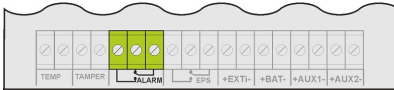
Fig. 10. Technical output ALARM.
