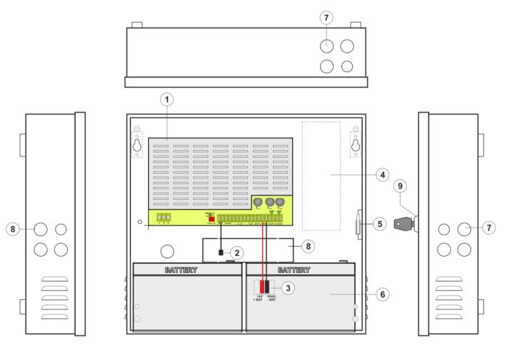
Fig. 3. View of power supply based on EN54C-2A7.
