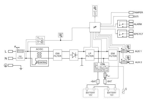
Fig. 1. PSU block diagram.
