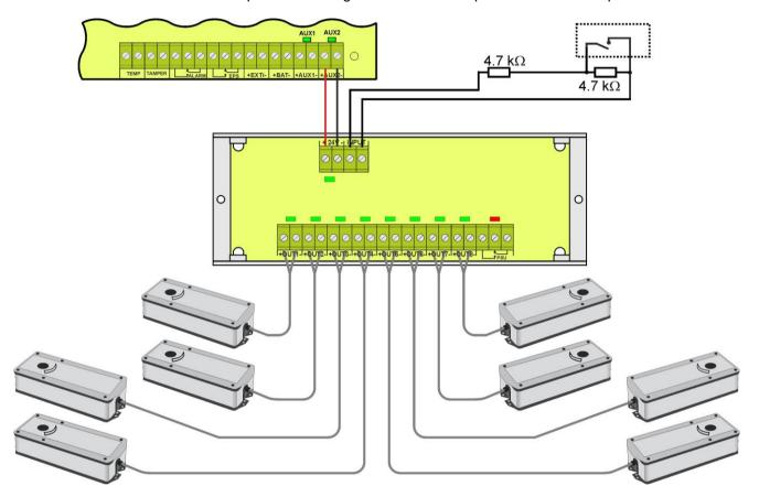
Fig. 13. Example of connection of the EN54C-LS8 sequential module with actuators with return spring.
