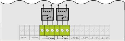
Fig. 7. Electrical diagram of relay outputs.
