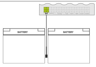
Fig. 14. Mounting of the temperature sensor.
