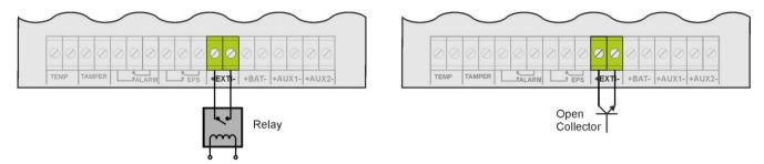
Fig. 10. Connections to the EXTi input.
