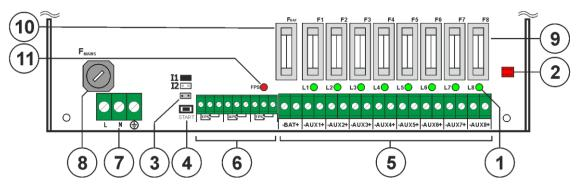
Fig. 2b. View of power supply module HPSDCG2-12V8x1A
