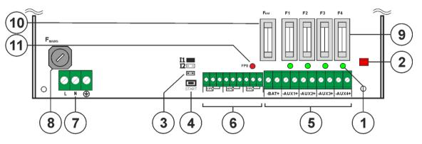
Fig. 2a. View of power supply module HPSDCG2-12V4x1A
