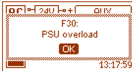
Fig. 14. Information that power supply is overloaded.
