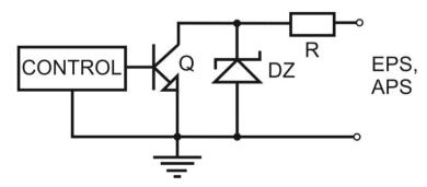
Fig. 4. Electrical diagram of OC outputs.
