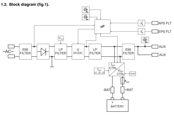
Fig.1. Block diagram of PSU.
