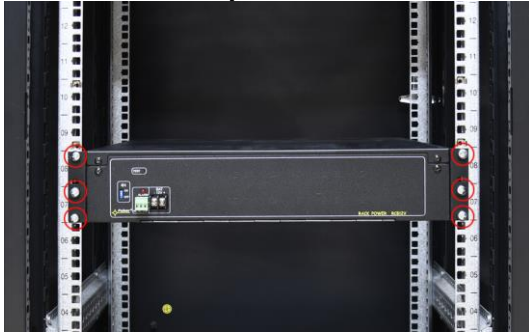
Fig. 3 Mounting the controller in a RACK cabinet.
