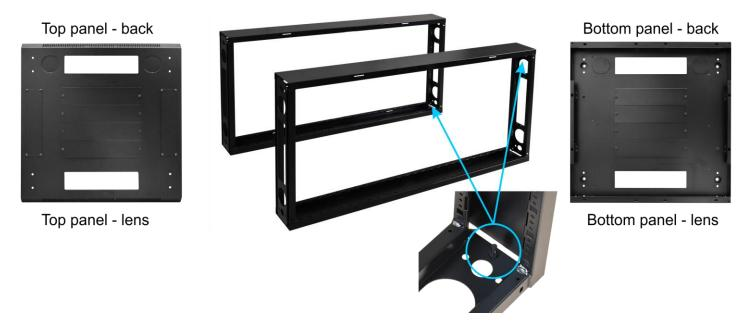
**5.2)** Mount the top plate and bottom plate to the left and right frames of the RACK cabinet, respectively. Use M8X12 Head Cap Screws with M8 nuts (16pcs). Screw the cabinet **wheels** and **legs** to the bottom plate of the cabinet.
