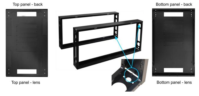
**5.2)** Mount the top plate and bottom plate to the left and right frames of the RACK cabinet, respectively. Use M8X12 Head Cap Screws with M8 nuts (16pcs). Screw the cabinet **wheels** and **legs** to the bottom plate of the cabinet.
