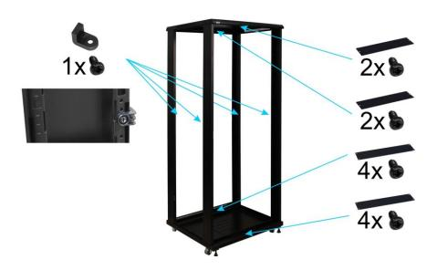
5.4) Mount to frames (in front and back) cross profiles, distances and RACK profiles as shown below.
