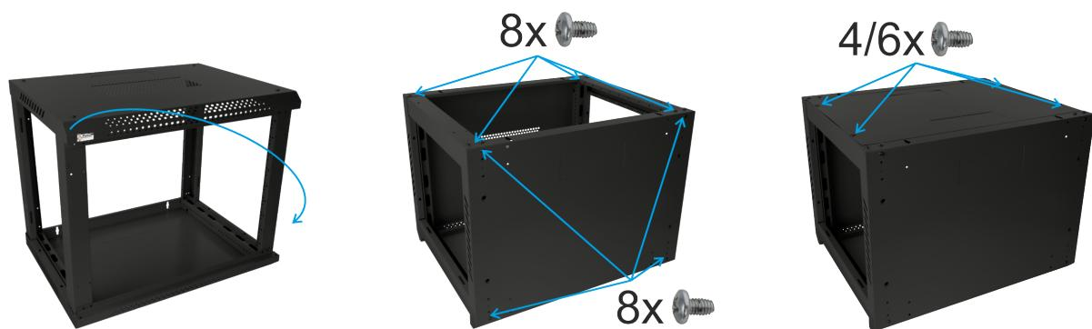
Lay the cabinet on its side and mount the RACK profiles with 4 screws (repeat the same process by laying the cabinet on the other side).
