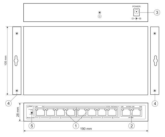
Fig. 2. The view of the switch.
