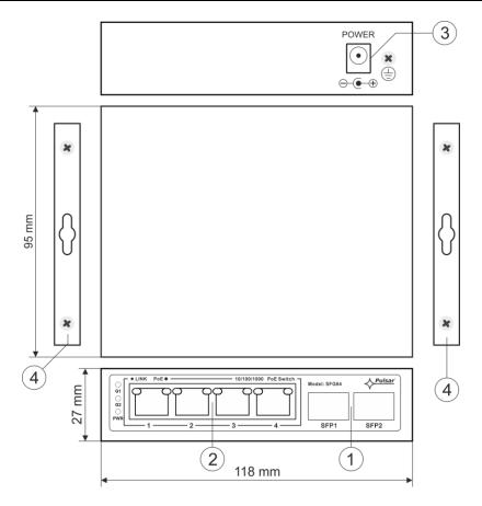
Fig. 2. The view switch'a.
