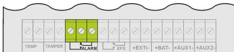
Fig. 7. Sortie technique ALARME.
