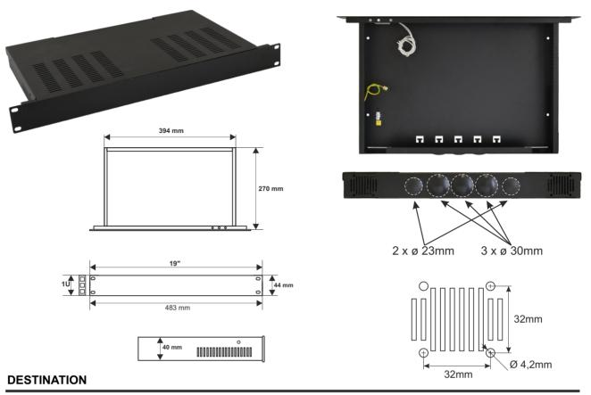
Due to its design, the ARAD1S enclosure is intended for mounting inside RACK 19" cabinets. This general-purpose enclosure may serve as an auxiliary element for integrating CCTV, AC, I&HAS, RTV, LAN systems in RACK 19" cabinets. It is intended for mounting alarm control panels, AC controllers, power supply units, batteries, etc.
