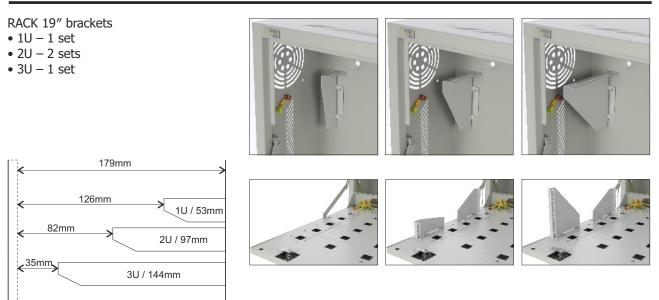
Distances inside enclosure after mounting 19' rack profiles, 179mm distance: hinged front door - bottom of the enclosure
