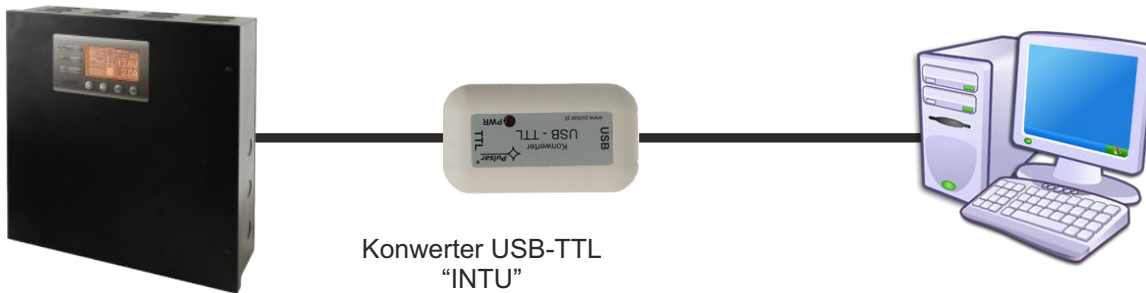
USB-TTL communication using the USB-TTL „INTU” interface.
