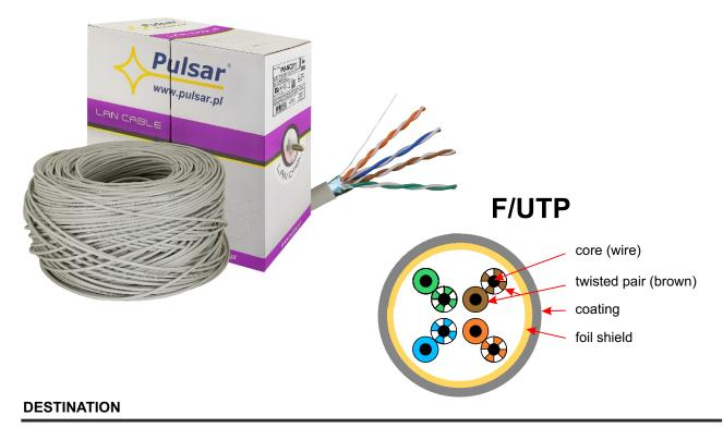
PU-NC211 is shielded twisted pair wire F/UTP, category 5e for data and power transmission (PoE). It can be used in many systems, i.e. ICT systems, IP video monitoring systems (especially recommended for IP PoE systems), but it will also work well in HD digital closed-circuit television systems (CVI, TVI, AHD). Cable is intended for professional installations inside buildings and complies with the EN 50575 (CPR) standard.
